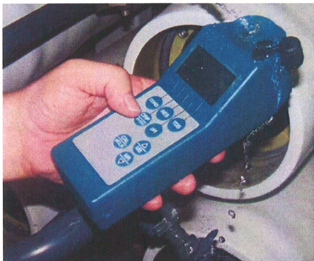
Figure 2: A simple handheld instrument that makes ORP measurements can be used to screen for tolerable levels of free chlorine and comply with membrane manufacturer's specifications.
