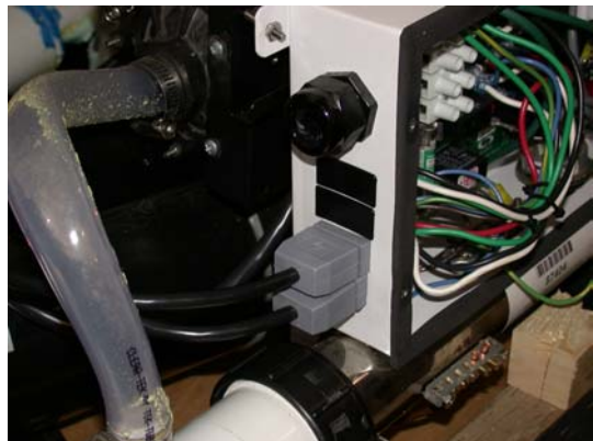
Installed J&J connector Figure 7
