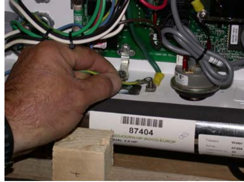
Attach ground ring securely Figure 9
